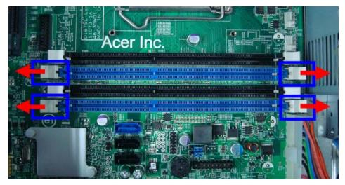
2. Insert the memory module into the DIMM1 slot (1) and then press it down until it clicks into place (2).
